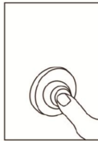
If the overload protector pops up due to low voltage or abnormal power connection during grinding, please check and troubleshoot first, then press the protector for normal use.
