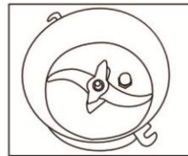
After loosening the nut, remove the spacer/gasket and the top two blades.
